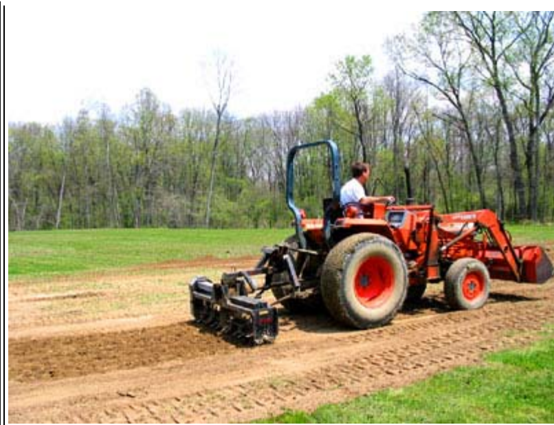
An operator aerates the entire field in preparation for adding a 3/8-in. deep layer of topdressing.
