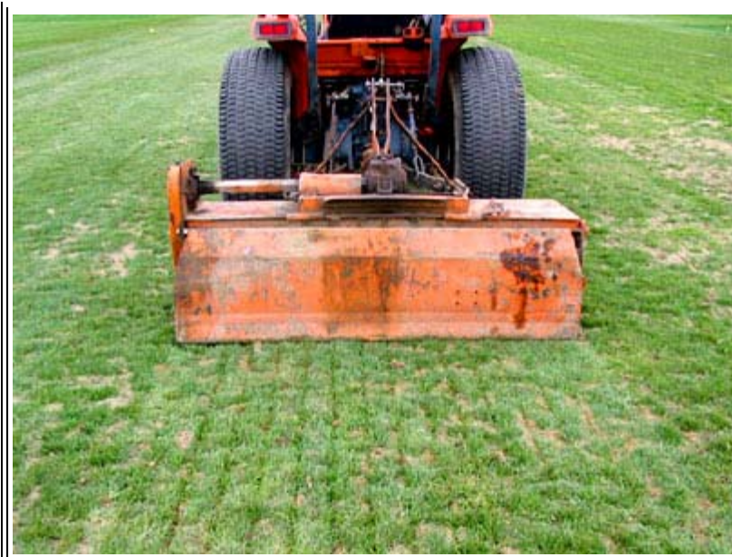
Slit seeding ensures good seed to soil contact.
