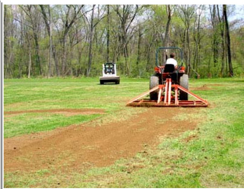
A 9-ft.-wide leveler fills in the divots and low spots to ensure an even surface before seeding.
